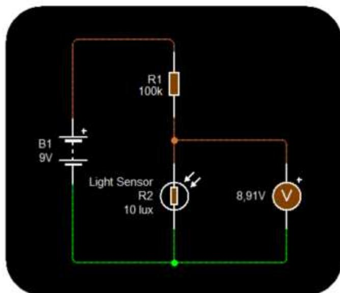
**Measuring Voltage**—Shows how a multimeter can be used to measure the voltage level (or potential difference) between two points in an electrical circuit.
