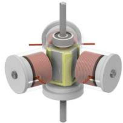
The current direction of coil and the magnetic field direction
