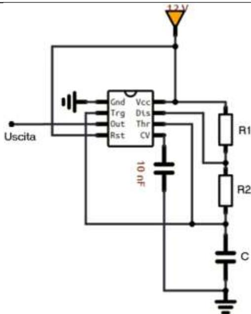
$$T = T_L + T_H = (R_1 + 2R_2)C \ln 2$$
